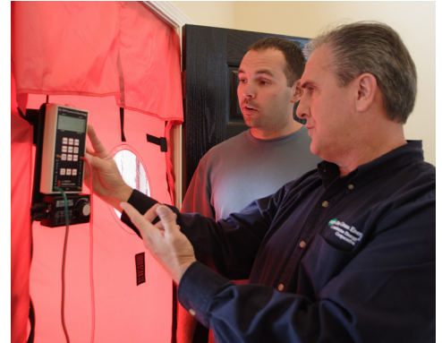
A blower door test can show where your home is in need of weatherization.
